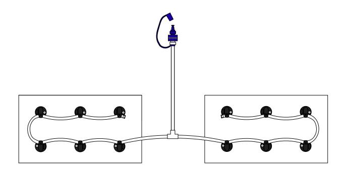
This is a guide to installing a 12 cell basic kit. The diagram(s) above show the most common configurations. Make sure tubing clears battery cables and all obstructions.
