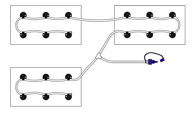
This is a guide to installing a 18 cell basic kit. The diagram(s) above show the most common configurations. Make sure tubing clears battery cables and all obstructions. Only water batteries after charging
