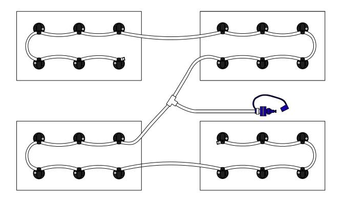
This is a guide to installing a 24 cell basic kit. The diagram(s) above show the most common configurations. Make sure tubing clears battery cables and all obstructions. Only water batteries after charging
