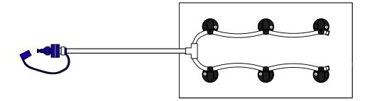
This is a guide to installing a 6 cell basic kit. The diagram(s) above show the most common configurations. Make sure tubing clears battery cables and all obstructions. Only water batteries after charging
