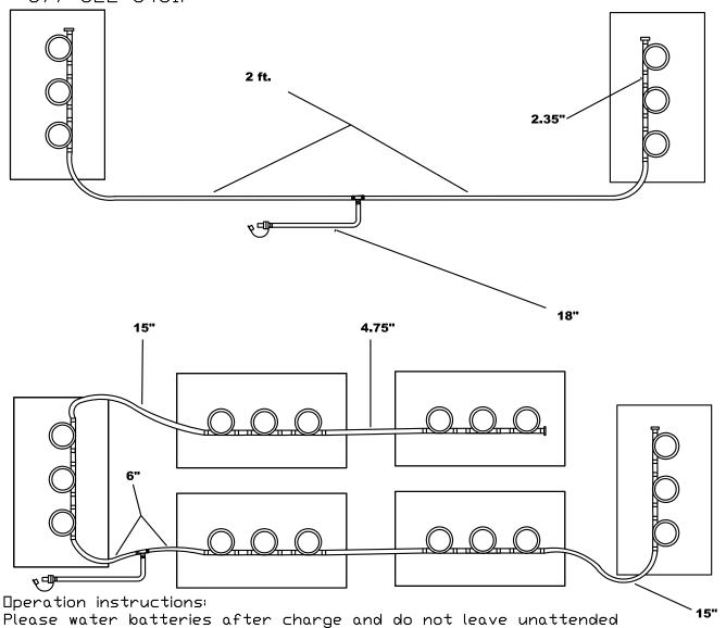
Connect the Delivery system (2 1/2 gallon tank, direct fill link, or direct fill gun) to single point on kit. Simply pull back on female quick connect and insert into male quick connect. When flow indicator stops spinning or all indicator eyes come to top of the plug, disconect quick connect
