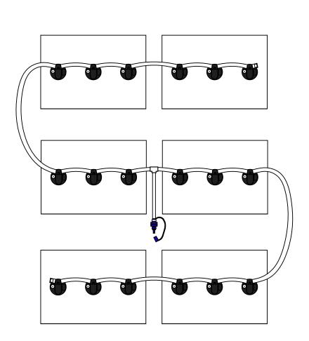
This is a guide to installing a basic kit. The diagram(s) above show the most common configurations. Make sure tubing clears battery cables and all obstructions. Only water batteries after charging
