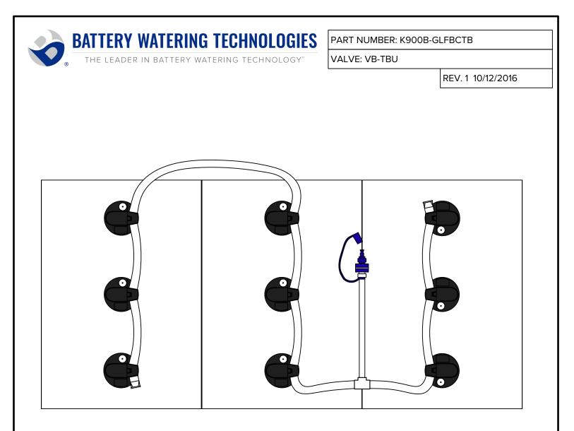
This is a guide to installing a basic kit. The diagram(s) above show the most common configurations. Make sure tubing clears battery cables and all obstructions. Only water batteries after charging
